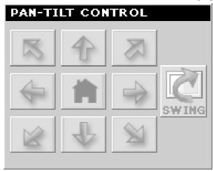
When you connect a pan/tilt camera, the system will detect the camera's function automatically and the PAN-TILT CONTROL buttons will become functional. Otherwise, these buttons are displayed as gray out buttons.
